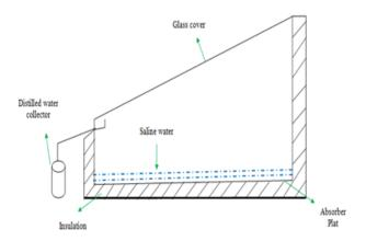
Figure 1: Schematic diagram of conventional solar still
