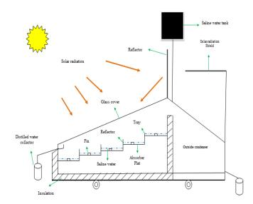
Figure 3: Modified stepped solar still schematic diagram.
