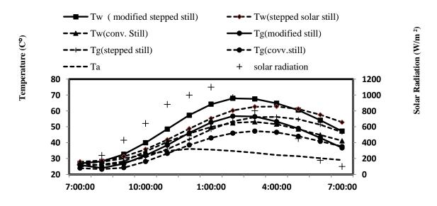
Figure 4: The hourly temperature variation and solar radiation for modified stepped solar still, stepped solar still without modification, and conventional solar still
